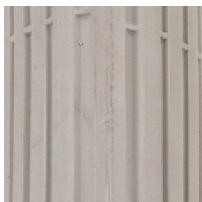
Tire for power wheelchair - profile: longitudinal grooves
