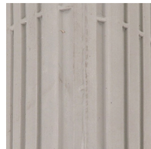
Tire for manual wheelchair - profile: longitudinal grooves
